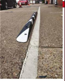
The Kerb Orca has 150mm wide modules, Middle (1000mm long, 11kg) and End (1000mm long, 9kg) with moulded in markings.
